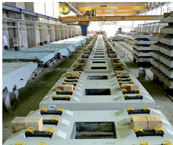
Series production at the concrete factory: track support plates for the slab track system
